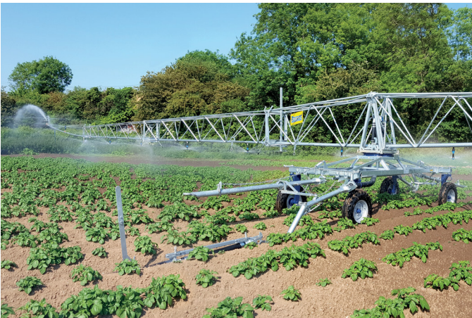
The pump is started, the hosereel is actuated and the boom begins to irrigate.
