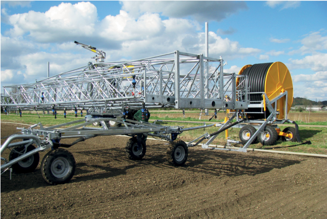
The boom is towed to the field where it is connected to the hosereel.
